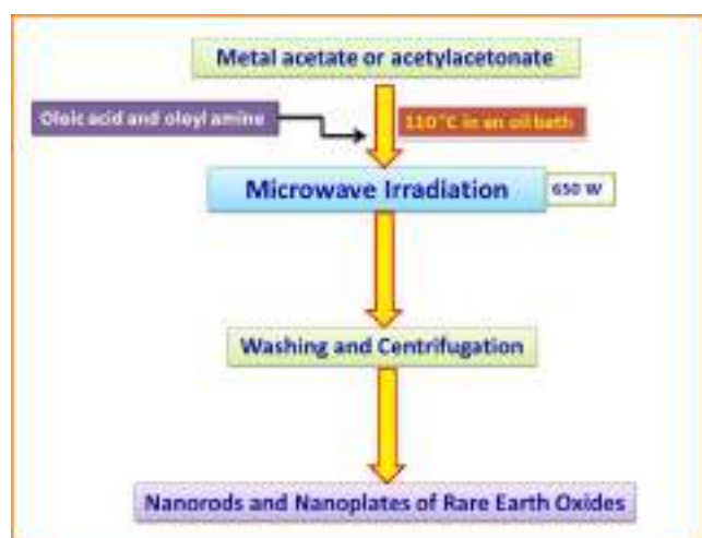
Fig. 6. Flow chart of microwave assisted synthesis technique.
